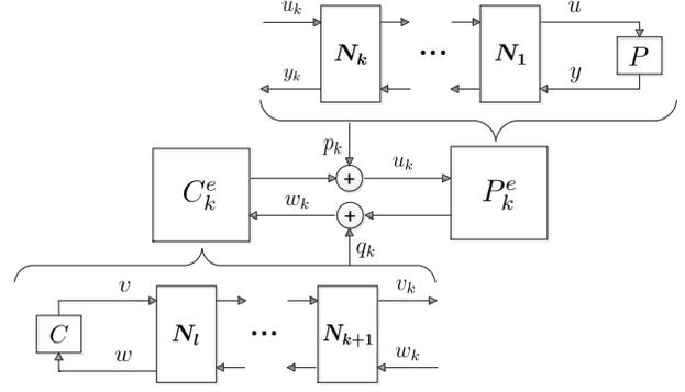
Fig. 5: Equivalent Plant and Controller
